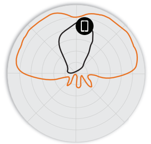
Figure 5 - T310d 5GHz Elevation Antenna Patterns
